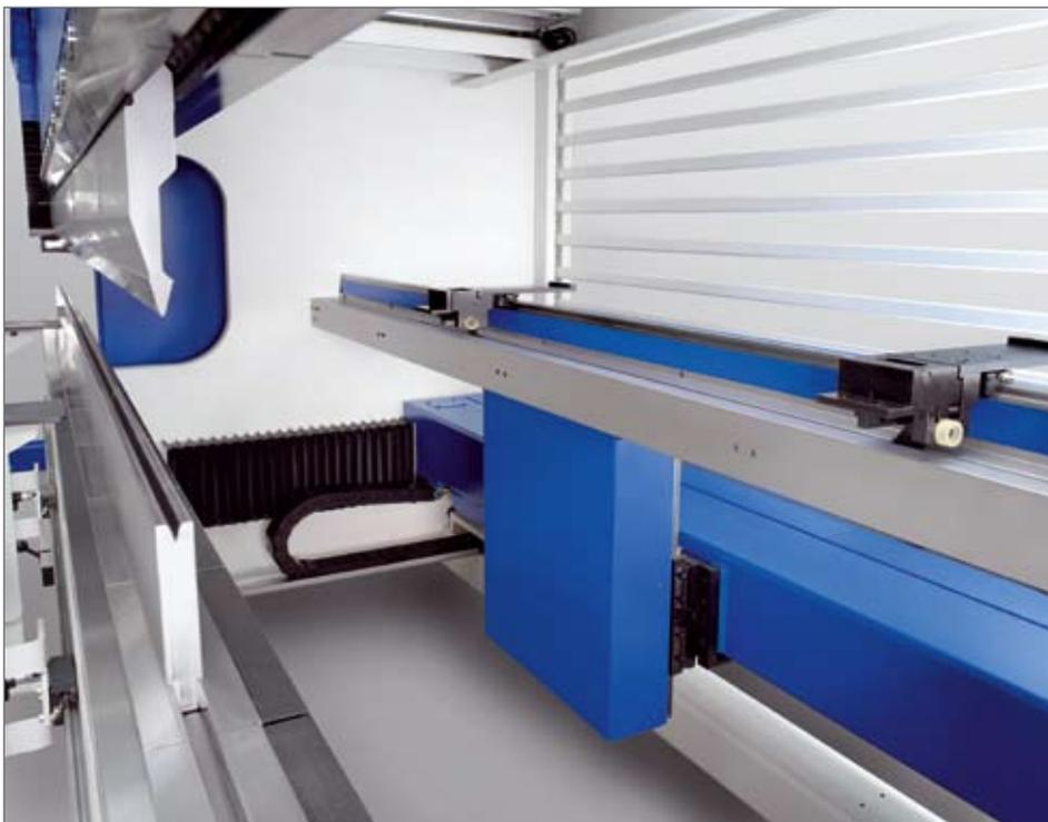
The position of the back stop fingers for the standard 2-axis system can be freely programmed in the X and R direction. The operator manually moves the stops in the Z direction where the push of a button is sufficient to move the stops in front of the bending line. After that, they can be safely positioned by hand and moved to the working position at the touch of a button.
