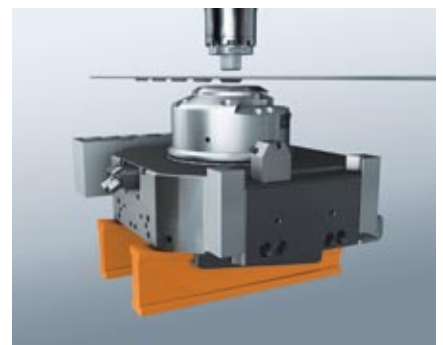
Scratch-free sheet positioning with the descending die.
