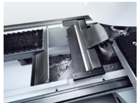
The sorter separates scrap from good parts.
