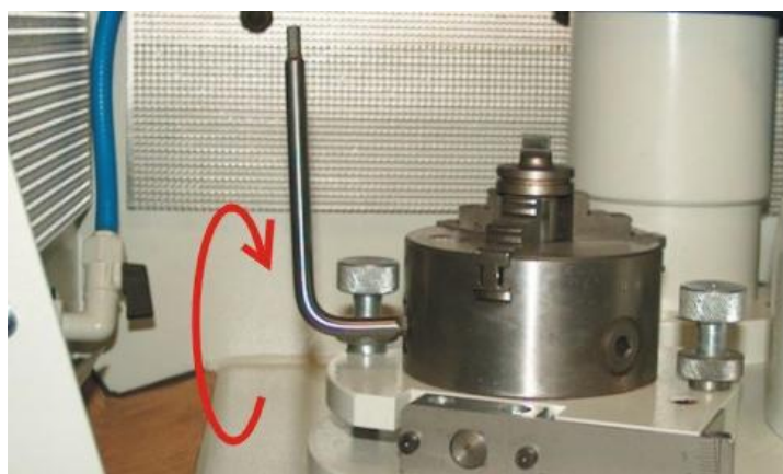
Aligning the punch: Simple alignment into the universal chuck with the hock wrench, which is included in the delivery scope.
